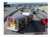
Barriers, Cones, Flares: Traffic cones provide additional visibility and act as a guide to divert traffic. Flares should be used when there is a need to increase visibility. TXDOT should be notified of extended lane closures. TXDOT has resources to help with traffic control and to notify the public.
